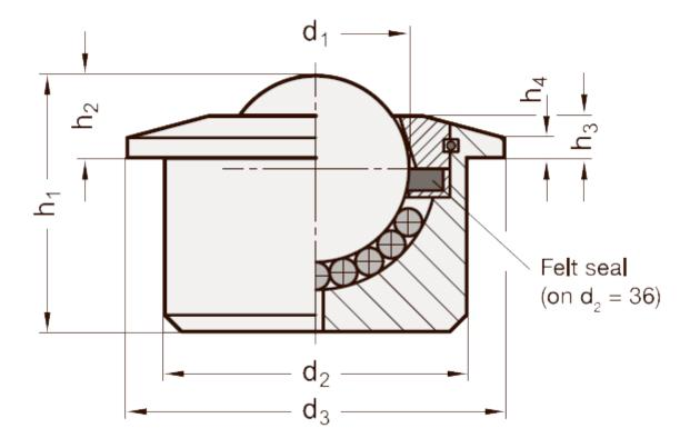
$$\begin{array}{lll} d1 & = 60 \\ d2 + / -0.08 & = 100 \\ d3 & = 117 \\ h1 + / -0.3 & = 77.5 \\ h2 + / -0.3 & = 30 \\ h3 + / -0.3 & = 15 \\ h4 & = 10 \\ Max load (N) = 13000 \end{array}$$
